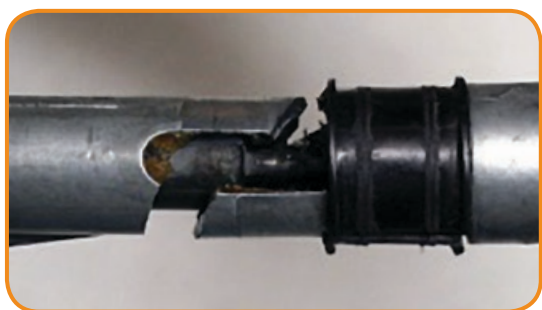
Competitor's unit is prone to breaking at high-stress point on shift tube
