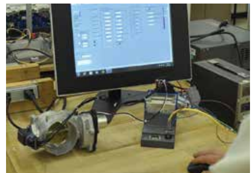
TechSmart® engineer performing TPS output test
