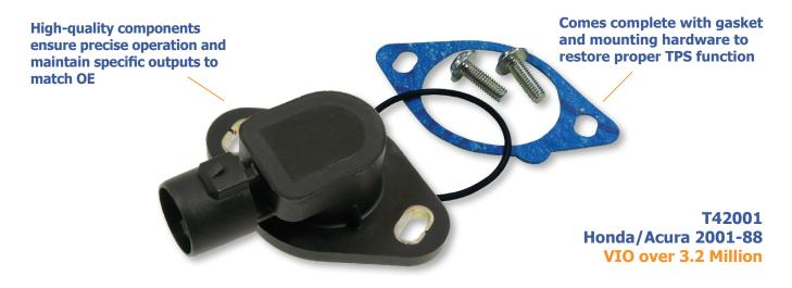
**TechSmart**<sup>®</sup> **Tip:** Once you remove the old rivets and install the new sensor using the included hardware, simply follow the OE service manual's TPS calibration procedure.
