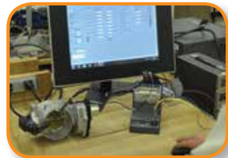
TechSmart® engineer performing TPS output test
