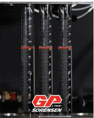
GP Sorensen® Injectors are tested and calibrated for consistency to optimize performance
